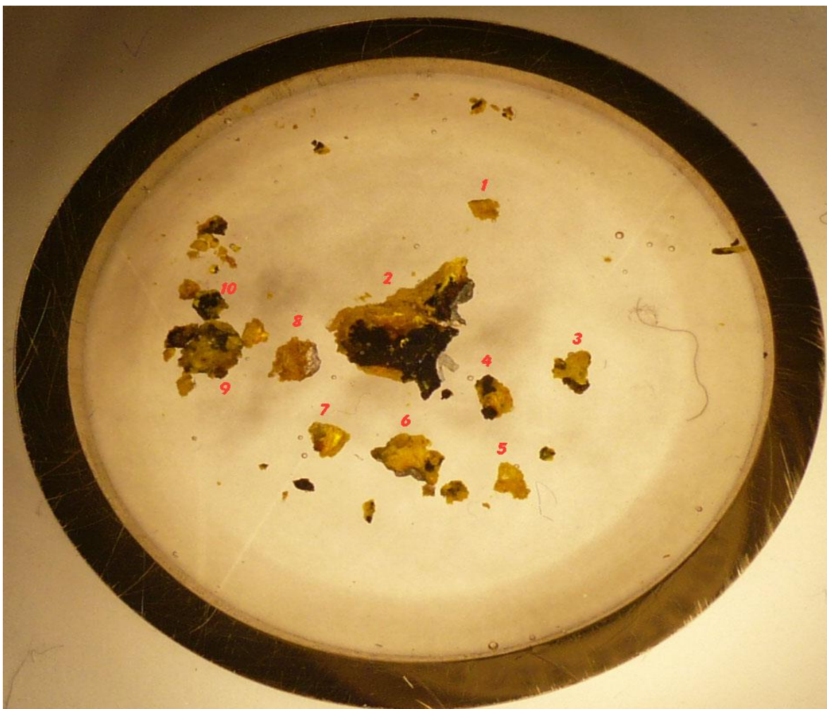
Figure 2-11: The prepared resin block for the EMA analysis, each number represents a different particle (as presented in Appendix C).
