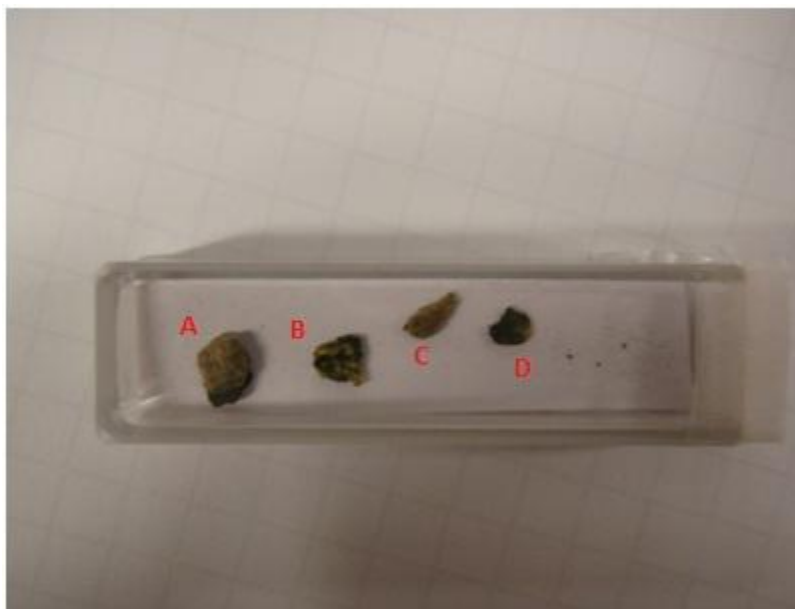
Figure 2-5: The prepared grains for Raman analysis from sample 8, Raman spectra have been measured for each of the grains A, B, C, and D as shown in Appendix A.
