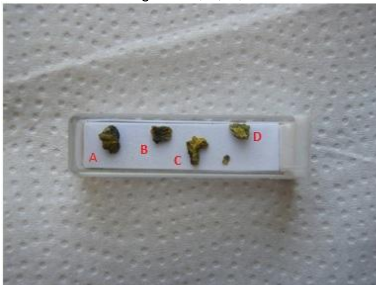
Figure 2-3: The prepared grains for Raman analysis from sample 4, Raman spectra have been measured for each of the grains A, B, C, and D as shown in Appendix A.
