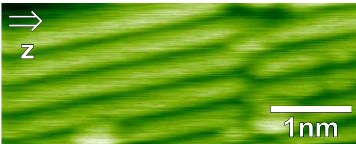
Figure 7.10: NC-AFM topography image of an anti-phase boundary perpendicular to the dimer rows.
