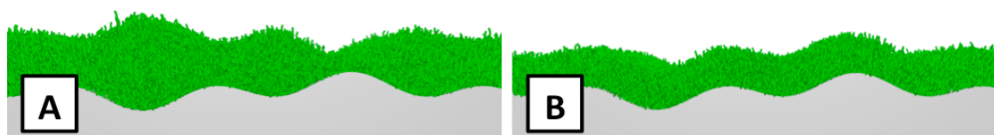
Figure 2.23: Schematic representation of an uncorrelated (A) and a partial correlated (B) polymer brush film.
