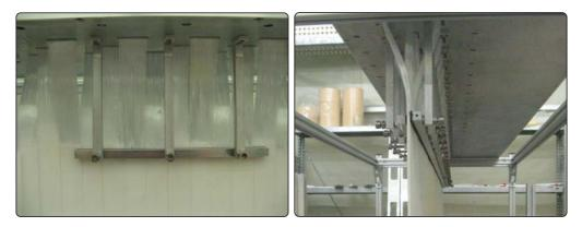
**Figure A.2:** Left. Photography of the crimping tool to keep the verticality of the fiber plane. Right. Side photography of the fiber plane showing how the crimping tool fits the plane.
