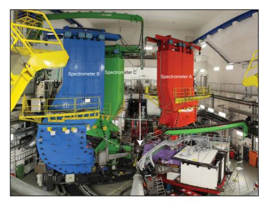
**Figure 1.4:** Panoramic view of the three spectrometers hall with the KAOS spectrometer showing the direction of the electron beam from MAMI (ca. 2009).
