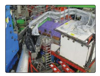
(c) General view of the KAOS spectrometer with fiber detector hodoscope installed (covered with black plastic). The hadron arm instrumentation is placed inside the radiation protection white walls at right.
