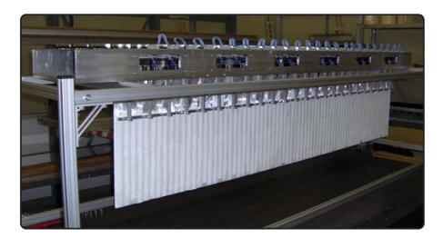
Figure 2.44: Photography of the fiber detector plane assembled in a supporting frame.
