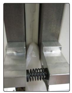
(c) Spread of the silicon layer applied in order to form a tiny layer.
