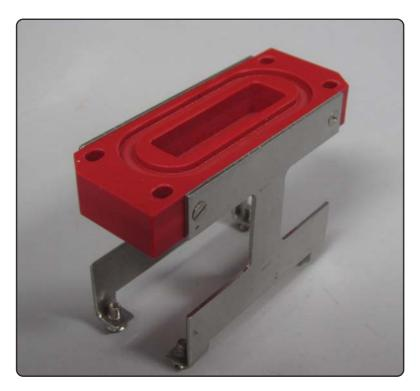
**Figure A.1:** Picture of the cookie with the clamping plates. It shows the groove for the O-ring for vacuum purposes. The hole in the middle is the place for glueing the fibers.
