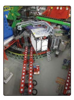
**Figure 1.6:** Right. Photography of KAOS in the platform at measurement position. Below the platform, in blue, can be seen one of the three supporting feet of the platform. Also below, is possible to see the end part of the position rails before retiring them. The white wall at right is a radiation protection for the detectors. Left. Photography of the platform rotated.
