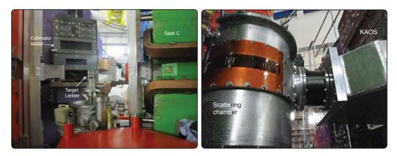
**Figure 1.7:** Left. Photo of the target position in the three spectrometer hall oriented from beam direction to beam dump. At left can be seen the collimator system at the entrance window of KAOS. In the center is the standard target ladder with different kind of solid state targets and at right the quadropole entrance of Spectrometer C. Right. Photo of the extension of the vacuum chamber of KAOS to the scattering chamber.
