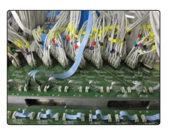
(b) Photography in detail of the triple boards with the signal cables already placed and the flat cables between the triple boards to power and control the HV bases of the MaPMT. The long blue flat cable is the main power and control cable from the HVSyS512 module
