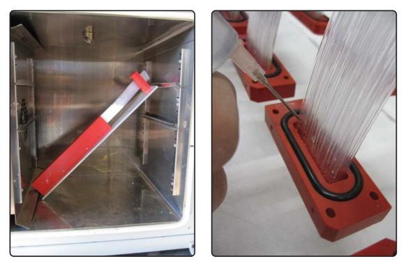
**Figure 2.36:** Left. Photography of the aluminium plate with the bundle into the air flow oven. The size of the oven allows to place three plates at time. Right. Detail of the application of the glue into the cookie with a syringe. The cookie has an O-ring placed.
