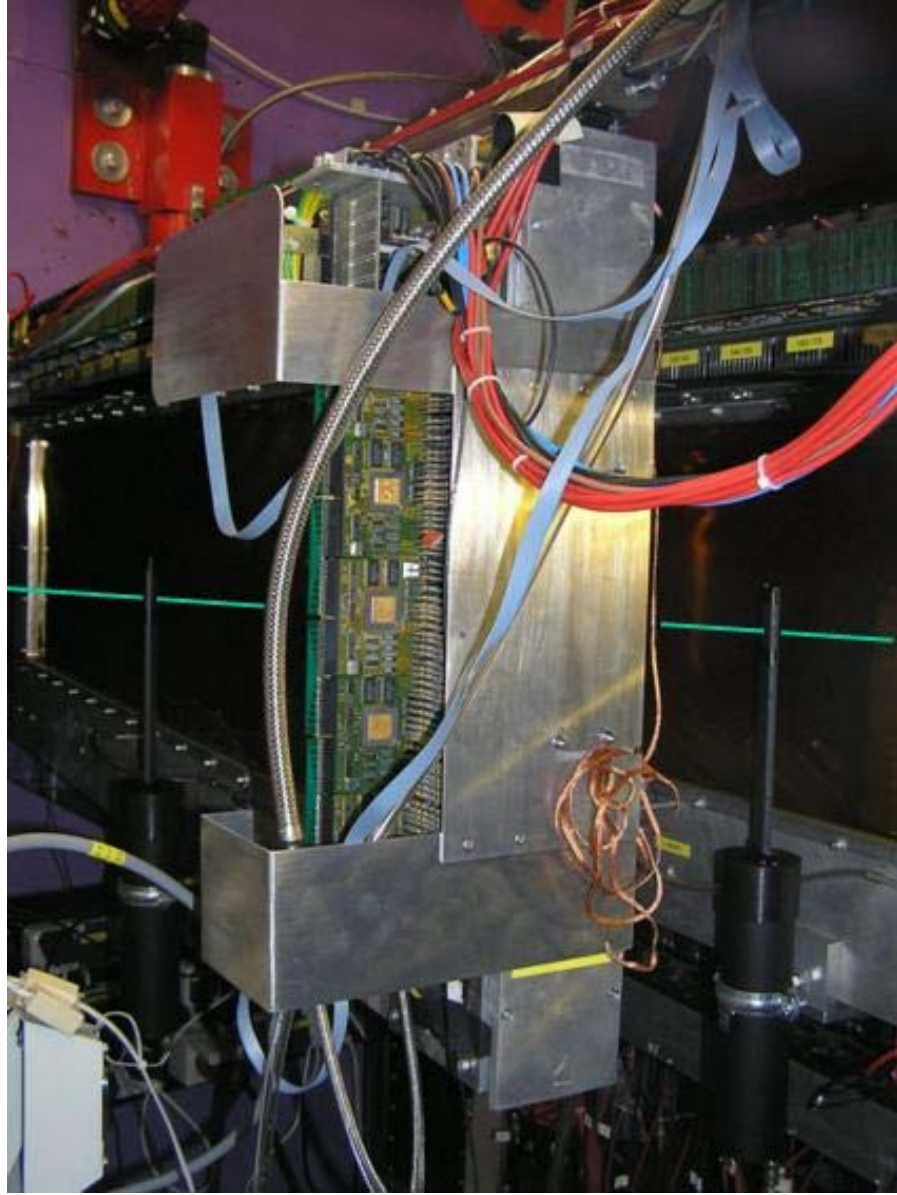
Figure 29: Efficiency counters placed in front of the MWPCs. A 3cm x 2cm x 0.5 cm piece of BC408 plastic scintillator vertically centered in the active area of the chamber is connected to a light guide 20 cm long and read out by a Hamamatsu PMT. Another twin counter is placed in front of MWPC L. A typical track crossing chamber M is shown in green. In order to define an event for the efficiency measurements, a hit in proper F and G paddles is also demanded to insure that MWPC L is also crossed before a possible decay
