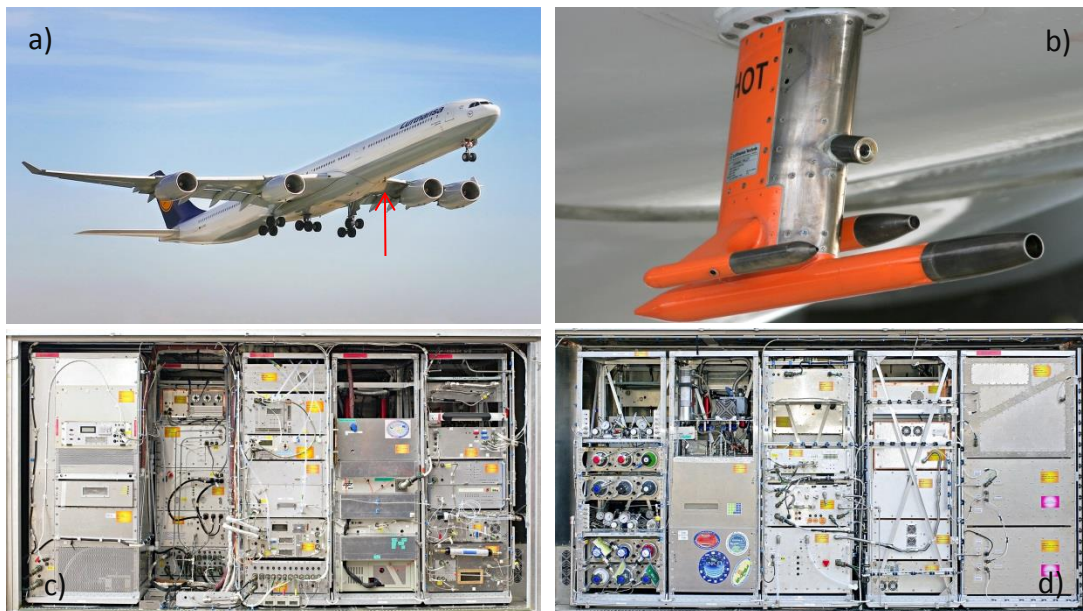
Figure 4-2: a) Airbus A340-600 with inlet system b) inlet system c) instrument container (front) d) instrument container (rear)
