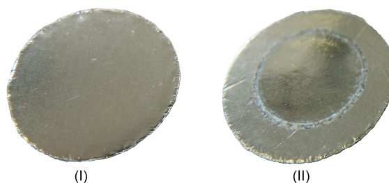
Figure 2.5 Left: Untreated tin foil. Right: Tin foil after multi-step electropolishing.
