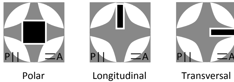
FIGURE 3.9: Maltese cross. Image of the Aperture diaphragm in the back focal plane, in the extinction condition, for the three different Kerr configurations. The positioning of the aperture selects the Kerr configuration. In order to probe magnetization pointing perpendicularly to the sample surface, the aperture has to be centered. The black areas indicate where the light is transmitted through the AD.
