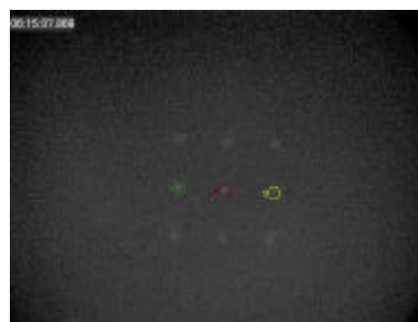
Figure 15: region measurements and SPFM image of the array1A after hybridization with 50pM target.
