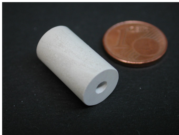
(a) Glass-ceramic blank as dielectric
