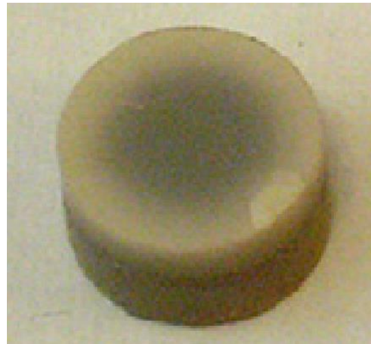
(b) Coring of sintered \text{TiO}_2 (1 h at 1500 °C) [PPW + 09]
