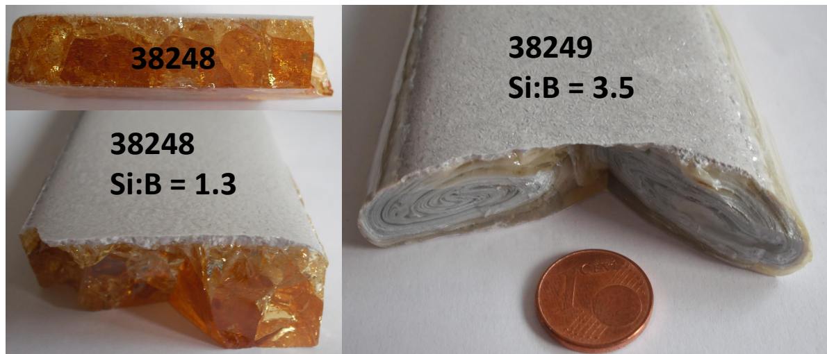
Figure 4.2: Comparison between a stable bulk glass (left) and a devitrified glass (right)
