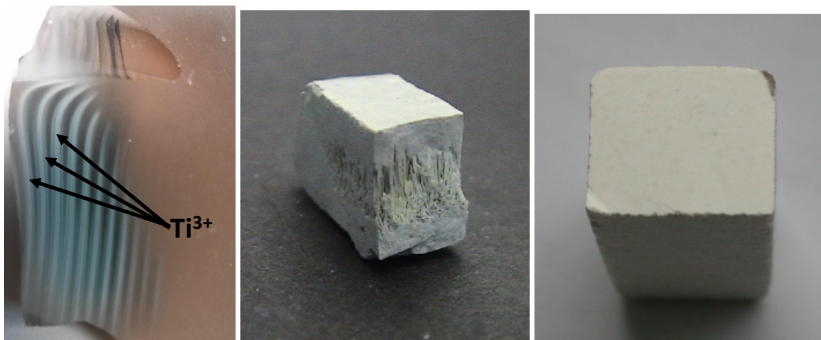
(a) Locally reduced ULE glass (blue Ti^{3+} striae) showing devitrification
