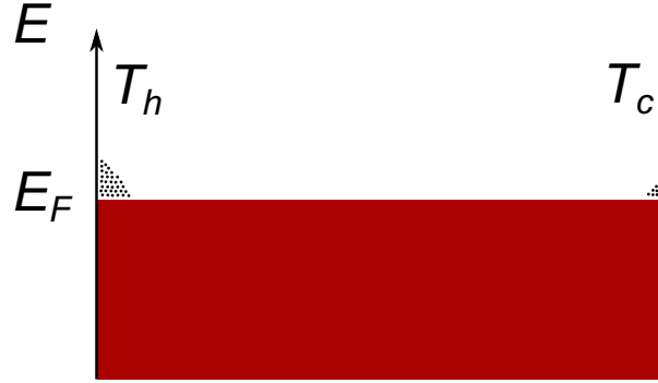
Figure 1.6.: Illustration of charge distribution in a metal
