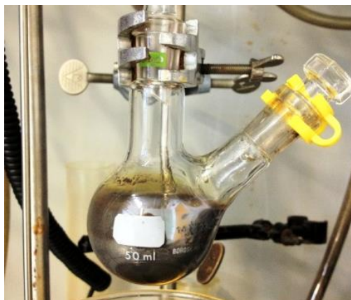
Figure 10. Silver mirror formed after the reaction for the synthesis of indolizine 78a
