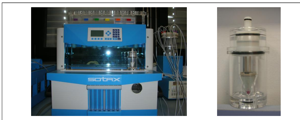
Figure 3-6 Left side: dissolution apparatus Sotax CE7 smart (USP apparatus 4). Right side: tablet dissolution cell equipped with liposome adapter.
