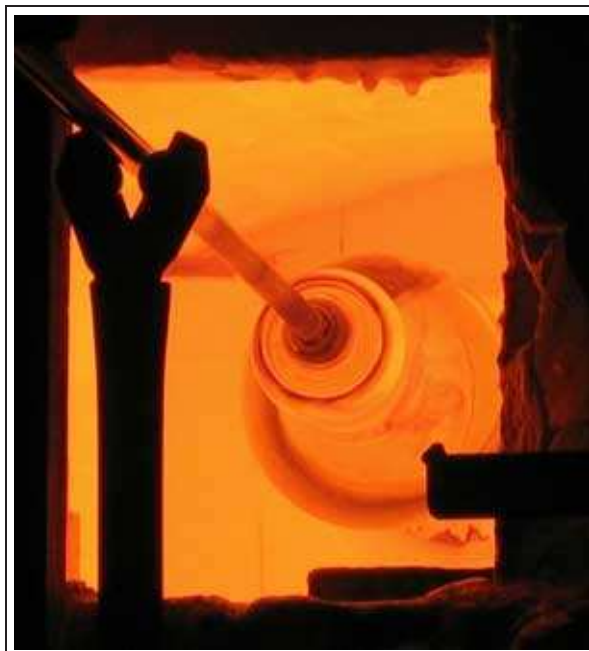
Figure 1.4: Molten silica being processed in a glass-work.
