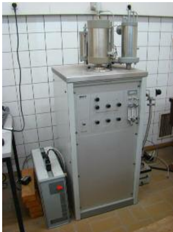
Fig. 3.2 Simultaneous thermogravimetry–differential scanning calorimetry (NETZSCH STA 429 CD).
