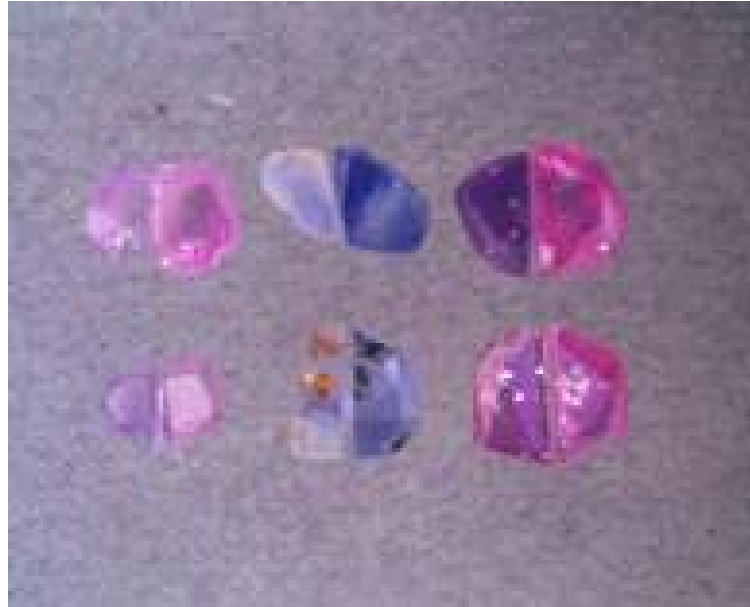
Fig. 1.3 Six corundum crystals from Ilakaka, Madagascar. The stones were cut in half for comparison. The right halves were annealed at 1750 °C (oxidizing conditions), whereas the left halves remain still in their original state for comparison (Häger, pers. Communication).
