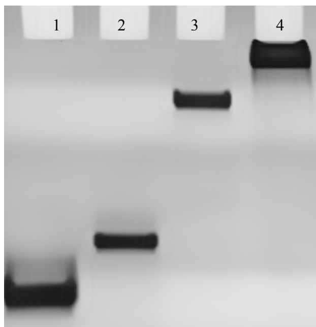
Figure 4.3 Lane 1 and 2 contain the triblock copolymers of ss DNA-PEG-ss DNA and ds DNA-PEG-ds DNA, respectively. Lane 3 and 4 contain the pentablock architectures of PEG(5K)-DNA-PEG-DNA-PEG(5K) and PEG(20K)-DNA-PEG-DNA-PEG(20K), respectively.
