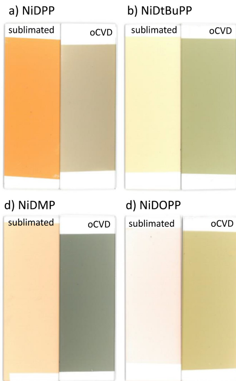
Figure S4. Optical image of the different coating obtained by simple sublimation (left) and oCVD (right) for each porphyrin on microscope glass. A) NiDPP b) NiDtBuPP c) NiDMP d) NiDOPP.
