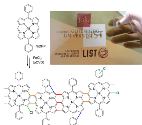
Scheme 2. The oCVD reaction of NiDPP yields a conjugated fused metalloporphyrin polymer with meso - \beta - meso (orange bonds) or \beta - \beta / meso - meso / \beta - \beta (red bonds) links between the monomer units. Potential side reactions, namely, cyclisation between a phenyl substituent and the porphyrin macrocycle (blue bonds) and chlorination of the porphyrin (green bonds), are indicated. The location of cyclisation and chlorination is not clear and merely representative. The inset shows an optical image of a bent transparent PEN foil coated by the greenish oCVD NiDPP film (top area of the foil) and the orange reference NiDPP film (bottom area of the foil).
