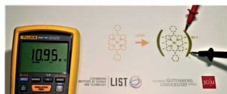
Figure 2. Optical image of the sublimed NiDPP coating (orange, left) and patterned oCVD NiDPP coating (green, right) deposited on paper. The green oCVD NiDPP coating displays electrical conductivity.
