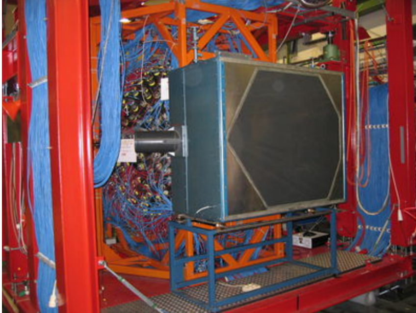
Figure 3.26: Picture of the Čerenkov detector covering the downstream opening of CB. On the left it is possible to see the photomultiplier tube. TAPS is absent in the picture because it was moved downstream for maintenance.
