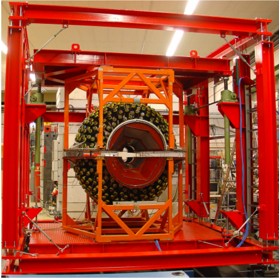
Figure 3.16: The Crystal Ball with photomultiplier tubes but without cables, during the installation at MAMI in 2002. Picture from [77].
