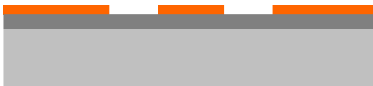
Fig. 18: Schematic sequence of process steps on wafer level for preparation of the coplanar wave guide: Step1 shows the full film deposition of the first \text{Al}_2\text{O}_3 insulation layer. In steps 2 to 4 the structuring of the coplanar wave guide with lift-off technique is depicted.
