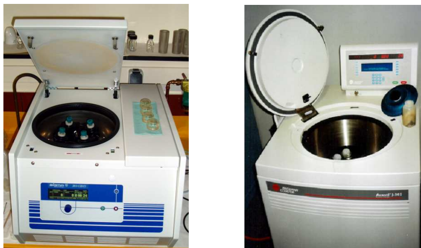
Figure 4.9: The table centrifuge used for \gamma\text{-Al}_2\text{O}_3 (left) and the ultra-centrifuge used for montmorillonite (right).
