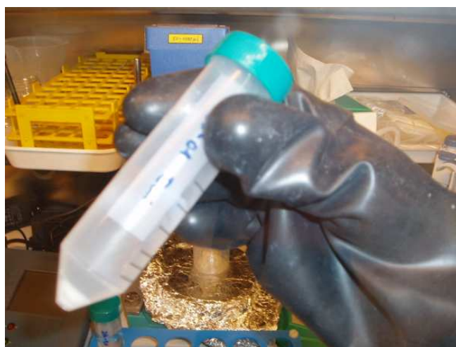
Figure 4.12: A sorption sample for EXAFS studies prepared in the glove box.
