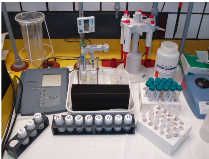
Figure 4.8: Manual pH adjustment of the \gamma - \text{Al}_2\text{O}_3 samples behind a lead brick. Suspension samples are kept in the green-capped vessels; for \gamma spectroscopy the supernatant is pipetted into the capsules placed in front.
