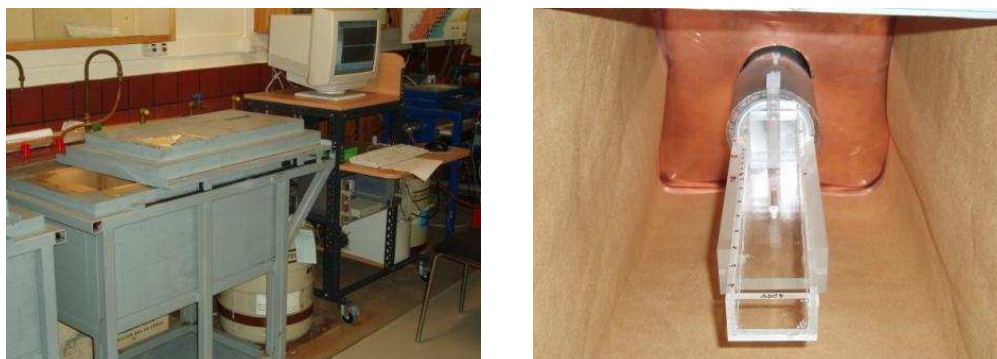
Figure 4.10: The \gamma detector at the Institute for Nuclear Chemistry, University of Mainz. For cosmogenic and laboratory background suppression, lead absorbers are placed around the apparatus. Left: general view; right: sample holder (front) and detector crystal with shielding (back).
