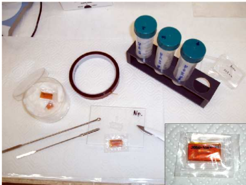
Figure 4.13: Preparation of the EXAFS samples. Insert: an EXAFS sample in an acrylic glass holder, girded with Kapton ® tape and twice heat-sealed in PE foil.
