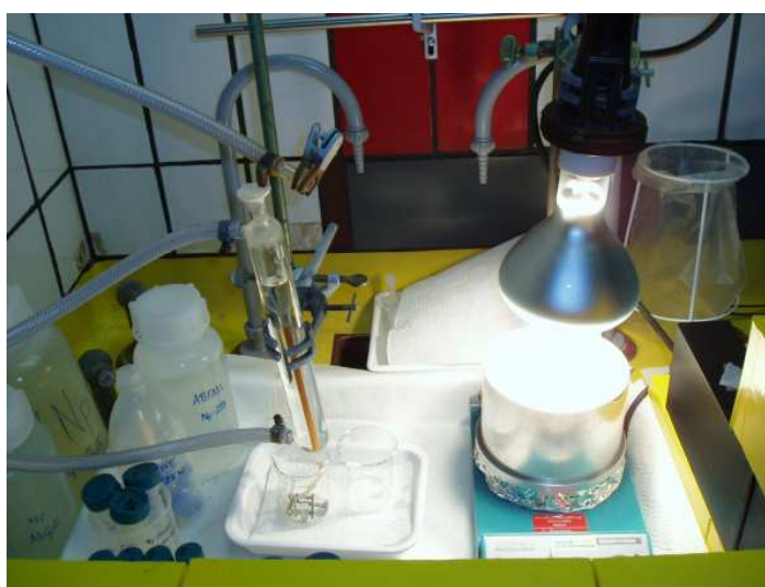
Figure 4.2: Cation exchange column and sand bath with infrared lamp.
