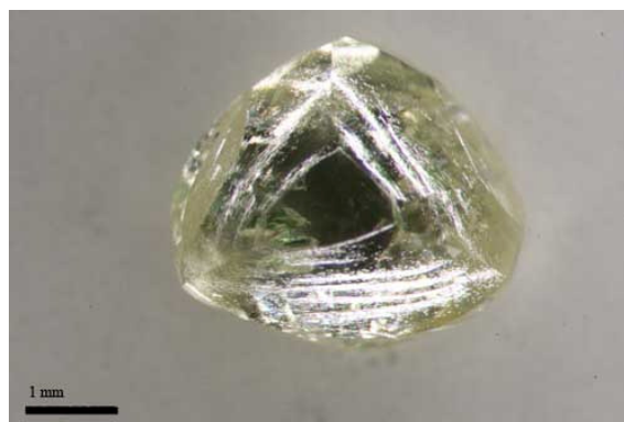
Figure 2.5 Octahedron with dodecahedral faces in sample DHF7 shows curved faces and round edges.
