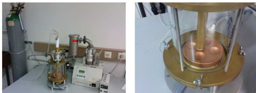
Figure 6.1: Home made arc melter set up with a water cooled copper plate including four indentations for three samples and a titanium sponge. The Ti sponge was used as oxygen gater during the melting process.
