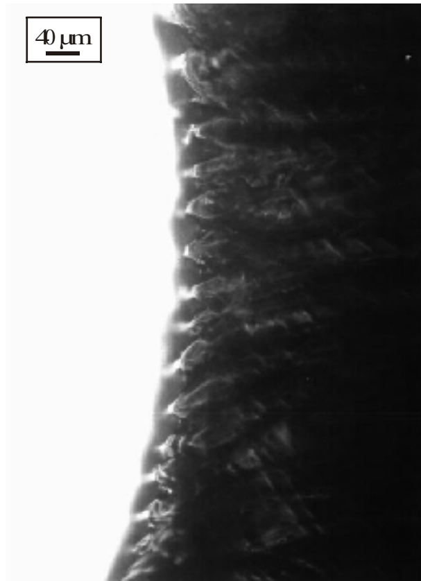
Fig. 3.11 Optical micrograph showing the faceting of the A-type grooves at the rim of the hole (experiment 53KAD5). The orientation of the sample could be inferred from the facets. Undersaturation was 0.2 \pm 0.2 °C, bulk stress was 4 MPa. The orientation of the face was close to \{111\} faces.
