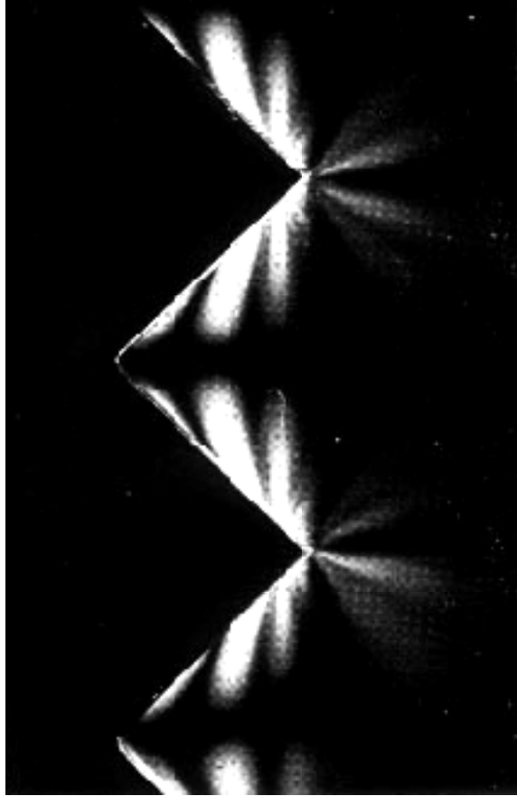
Fig. 3.13 Illustration of the localisation of the elastic strain in grooves made visible by photoelasticity in a Plexiglas model about 3 x 3 x 1 cm in size. Stress was applied vertically.
