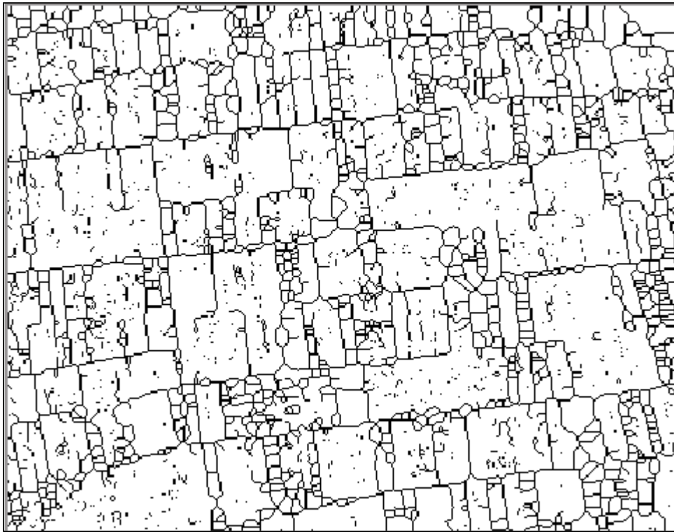
Figure 7-7-3 Result of Chen-Hsu algorithm: K = 1 , N = 3 , T = 20\%
