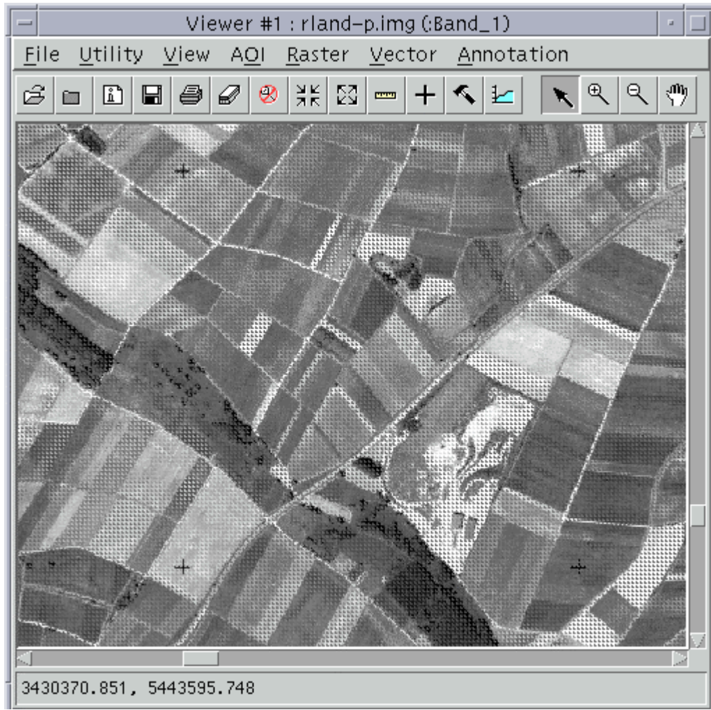
Figure 4-5 A subset of overlay of rectified panchromatic image and digital orthophotos
