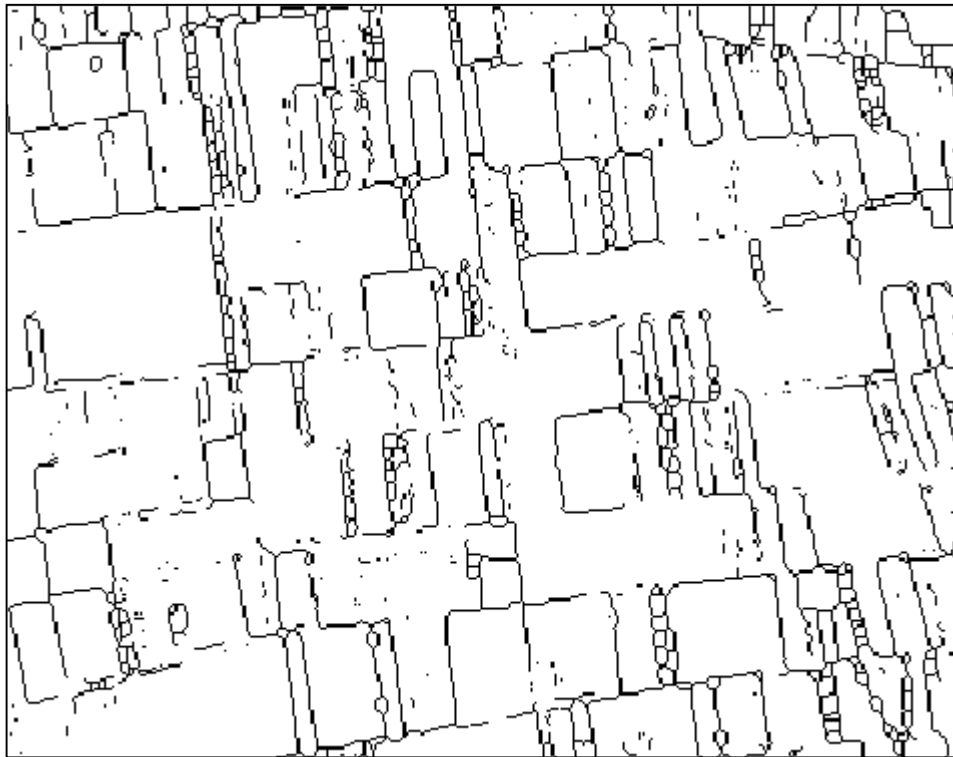
Figure 7-7-1 Result of Chen-Hsu algorithm: K = 1 , N = 3 , T = 10\%
