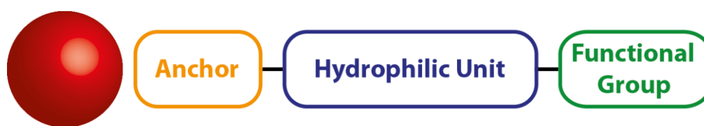
Figure 1.7.1. Schematic image of the ligand used in the fabrication of QDs for biological applications. 114
