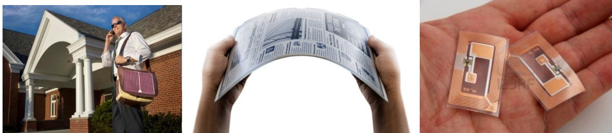
Figure 1. Examples of lunched applications based on organic electronics: paper thin, flexible solar panel providing enough power to charge a mobile phone (left); Electronic paper (middle); Roll-to-Roll printed rewritable memories on flexible substrate printed radio-frequency identification tag (right).
