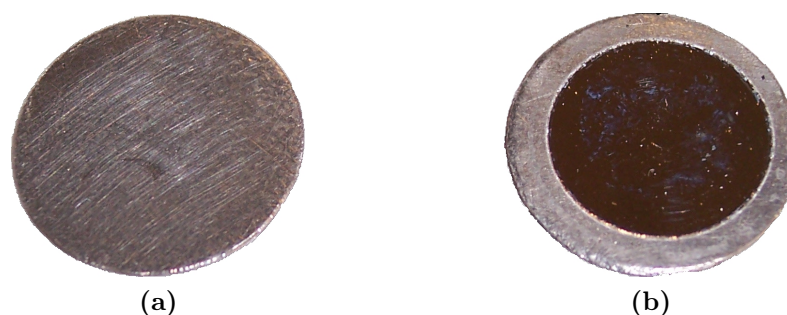
Figure 6.2: (a) Tin foil as-purchased from the manufacturer (after cutting to size) (b) tin foil after electropolishing.
