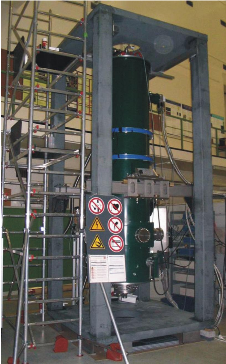
Figure A.5: Setup of the spectrometer aSPECT inside the anti-magnetic screen, a combination of construction steel (plates of cross-section 180 \times 180 \times 10 \text{ cm}^2 and thickness 10 cm) and ARMCO iron (pillars of cross-section 20 \times 20 \times 10 \text{ cm}^2 and length 400 cm). The shield provides a sufficient reduction of the exterior magnetic field (cf. Fig. A.6). Photograph taken from Ref. [1].
