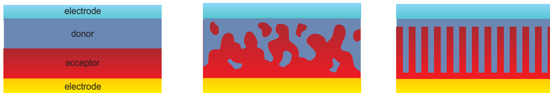
Figure 2.3: Examples of device architectures: bilayer heterojunction (left), bulk heterojunction (middle), and ordered, bulk heterojunction (right).
