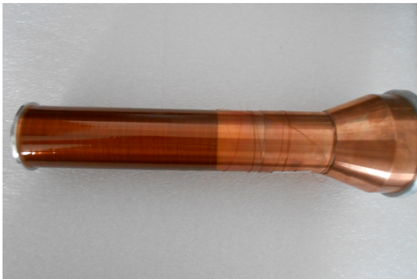
Figure 4.9: A picture of the longitudinal internal holding superconducting coil.
