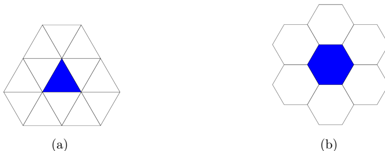
Figure 5.2: The topology of the crystals in a cluster. (a) is the Crystal Ball cluster of 13 crystals and (b) is the TAPS BaF 2 cluster. The crystal marked with blue is the crystal with maximum energy deposit, where the particle likely hit.
