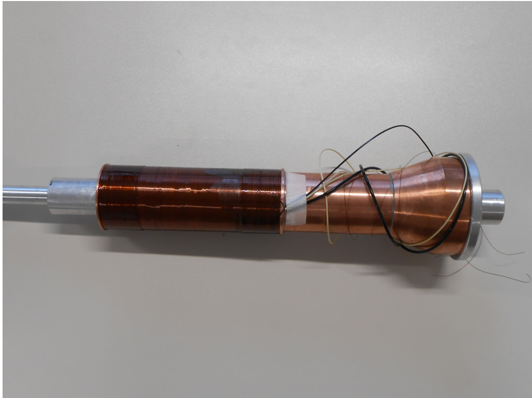
Figure 4.21: A picture of the completed internal superconducting polarizing magnet.
