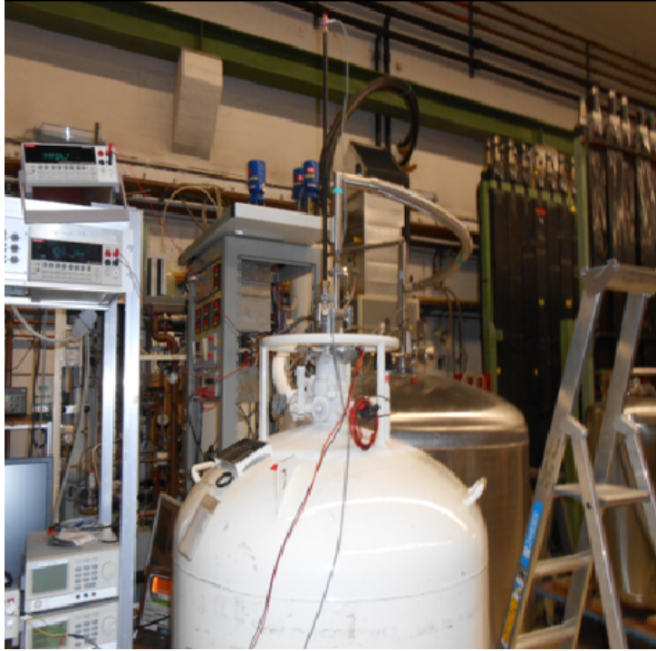
Figure 4.23: The internal polarizing magnet test setup.
