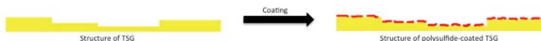
Figure 4.116: Scheme of the recreation of TSG structure by the adsorbed polysulfide (shown in red) (not drawn to scale).
