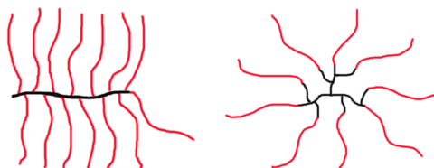
Figure 4.51: Scheme of PG-polysulfide copolymers with different architectures (red = polysulfide; black = PG) (left: brush copolymers from lin PG; right: star copolymers with hb PG core).
