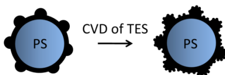
Figure 2.5: Sketch of coating raspberry particles with 5-25 nm sized silica nanoasperities making use of CVD of TES.
