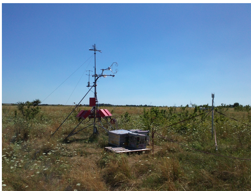
Figure 2.2: Setup of the instruments at the airfield Mainz-Finthen. On the left side the main mast is displayed with the sonic and the ozone sensors (red boxes), on the right side the weather station is on a second mast. The picture is taken in south-western direction.
