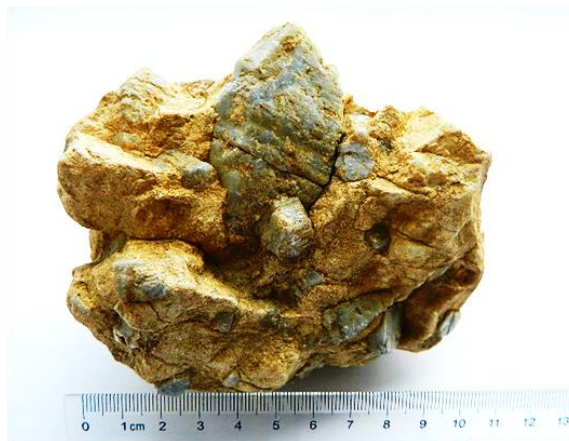
Figure 2.1.1.2.2: Sapphire crystals in polycrystalline of feldspar from an unknown source in northern Vietnam.
