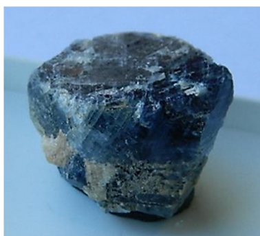
Figure 1.2.2.1: Parting along the rhomboheron \{10\bar{1}1\} in a Russian sapphire in this study. This sapphire is opaque blue and 20 mm in diameter.
