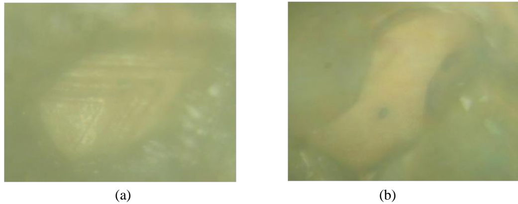
Figure 3.6.3: Goethite inclusions from Dak Nong (Vietnam) under reflection light: (a) A goethite crystal inclusion with twinning structures, (b) Goethite as inclusion containing a black graphite inclusion.
