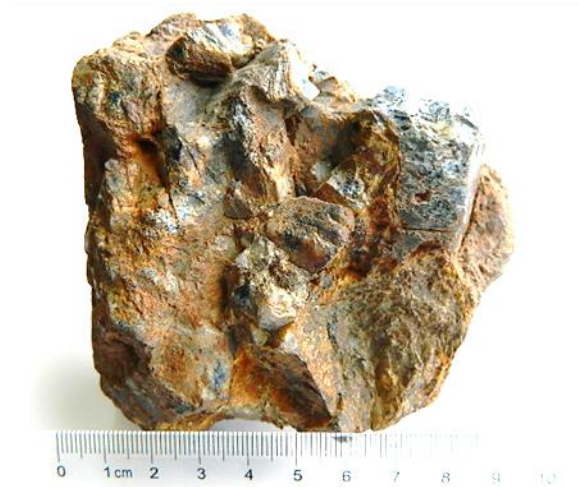
Figure 2.1.1.2.1: Sapphire crystals in a host rock from Quy Chau in the north of Vietnam.
