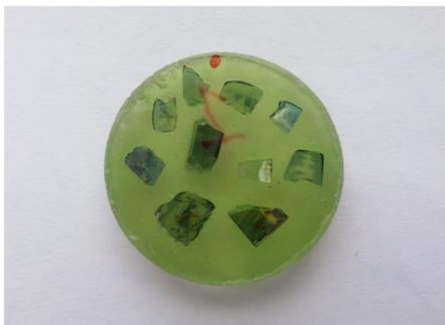
Figure 2.2.5: The samples are mounted in epoxy plugs.
