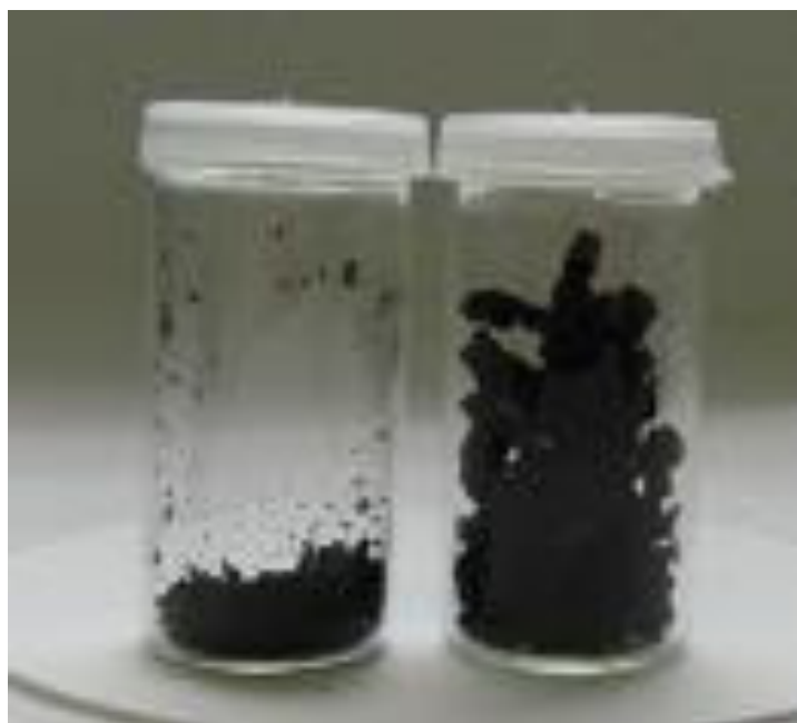
Figure 19. Left: graphene sheets from graphene oxide dried by rotary evaporator; Right: graphene sheets from graphene oxide foam by freeze drying.
