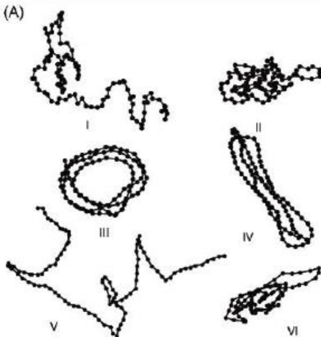
Figure 33. The typical conformations of polymer chains (I, random coil; II, molten globule; III, toroid; IV, rod; V, defect-coil; and VI, defect-cylinder) [7].
