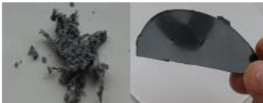
Figure 30. Left: the powder of graphene polystyrene composite. Right: the film of graphene polystyrene composite
