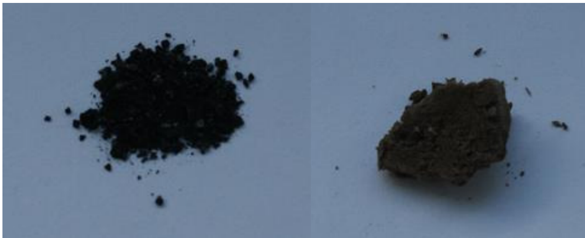
Figure 7. Graphene oxide Dried by rotary evaporator under vacuum at 50 °C (left); graphene oxide foam prepared by freeze drying (right).
