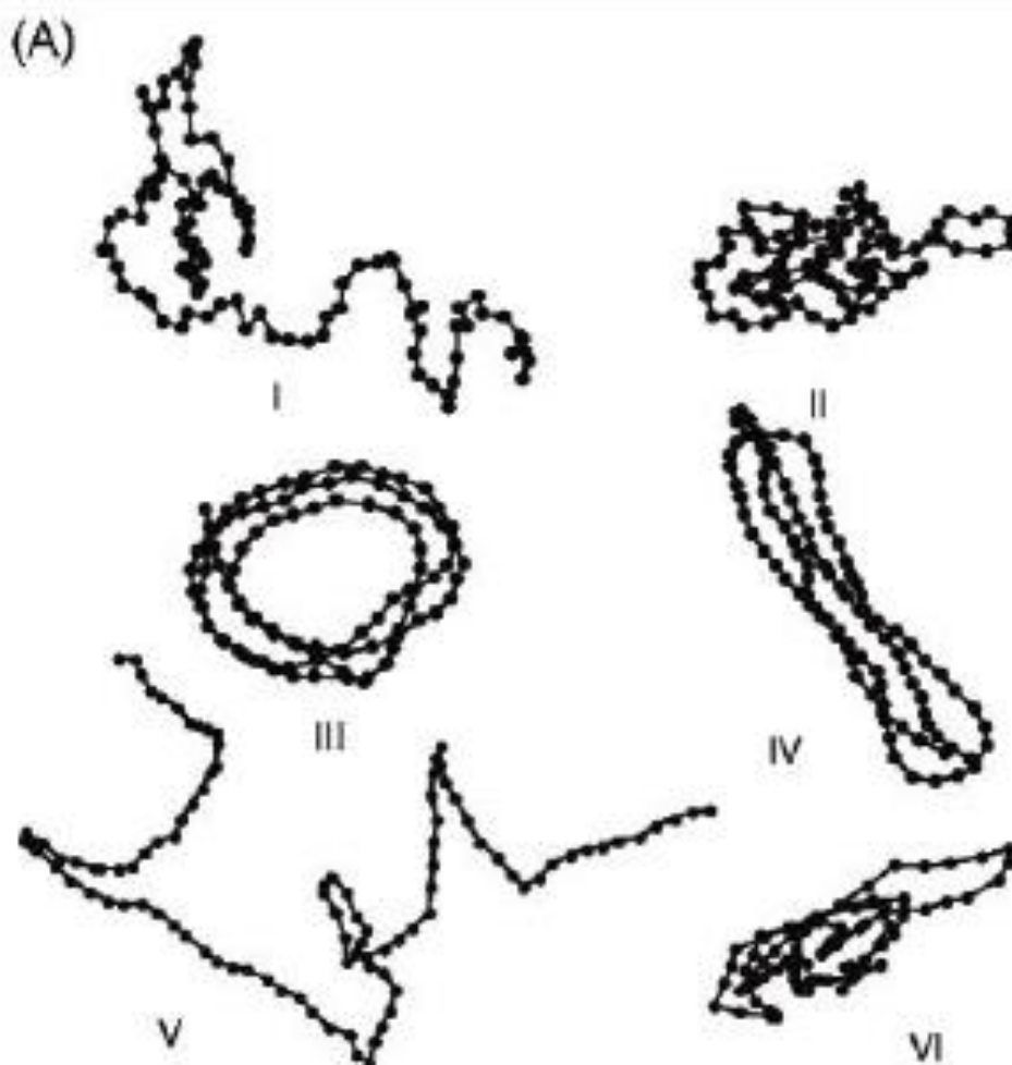
Figure 26. The typical conformations of polymer chains (I, random coil; II, molten globule; III, toroid; IV, rod; V, defect-coil; and VI, defect-cylinder) [7].
