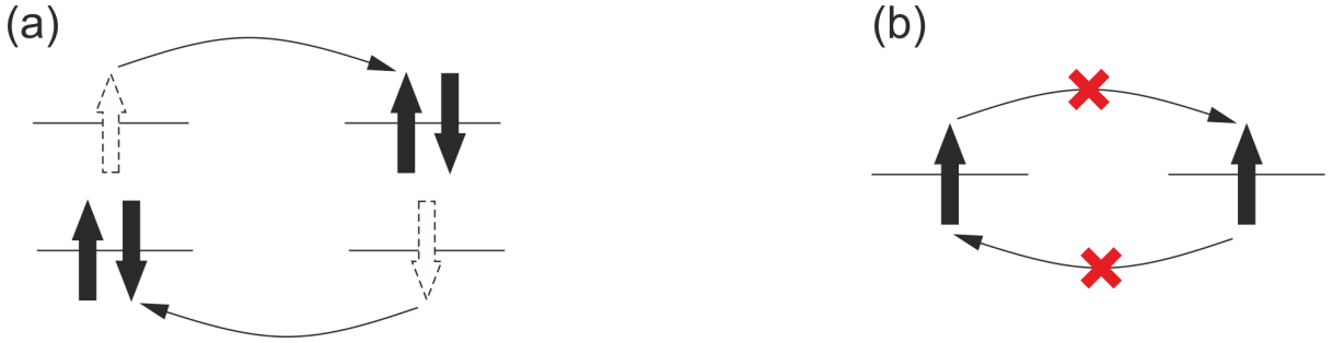
Figure 2.2: The states, which can be realized in a system of two atoms, each having a single unpaired electron. The spins of the electrons are (a) antiparallel and (b) parallel. The Pauli principle prevents hopping in (b).
