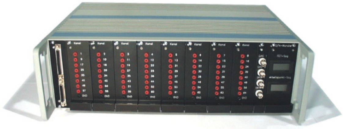
Figure 4-11. 64-channel main amplifier unit. On the frontside the 64 plugs for additional observation of the post-amplified signals can be seen.
