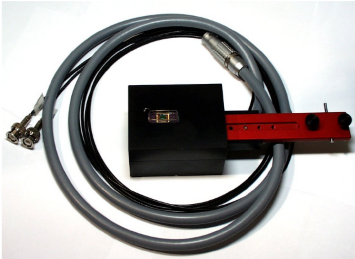
Figure 4-6 Preamplifier headstage for the backside contacted FET devices. The size of the housing and the principle of the amplification circuitry is similar to the standard FET preamplifier developed by Offenhusser et al. (1997), Sprosler et al. (1998) and Krause (2000).
