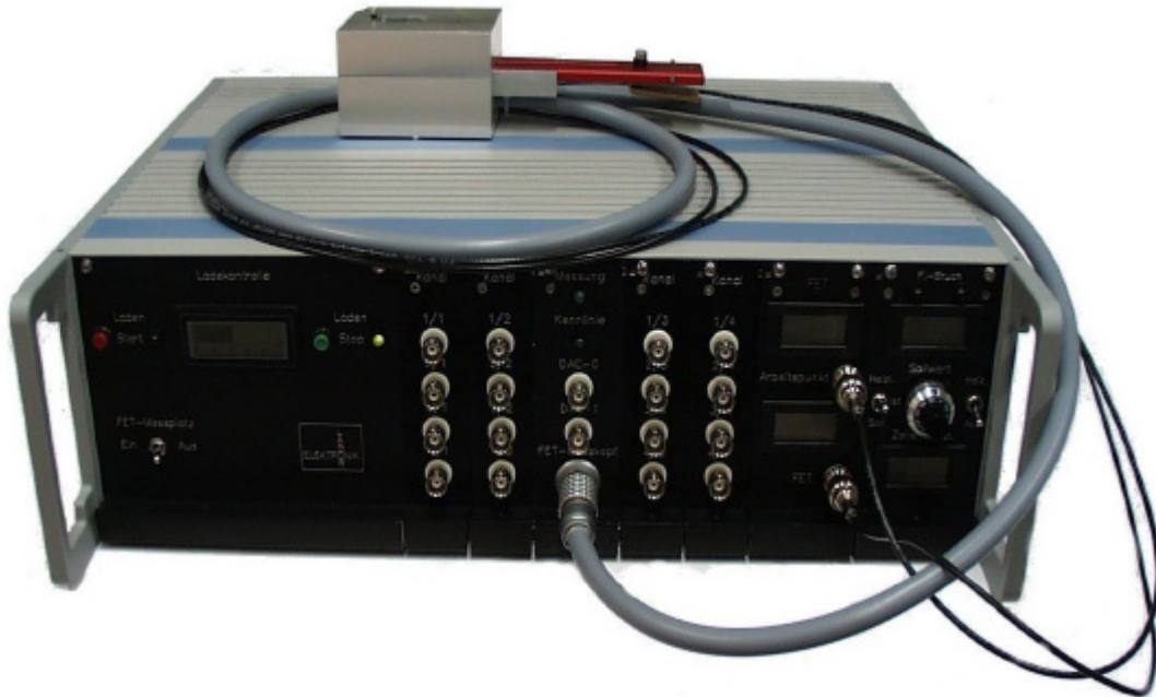
Figure 4-10 16-channel FET- and EGE-main amplifier unit. On the left side the plug-in unit for the battery supply can be seen. The middle part offers the possibility to connect a BNC-cable to each channel for external observation. Here the postamplified signals as they are read with the PCI 6110 data acquisition card (plug at the backside) can be observed. On the right side the heating unit can be seen.
