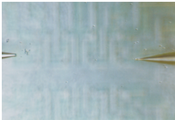
Figure 6-70 With two glass pipettes of the double patch-clamp set-up (Figure 6-71) gentle pressure was given to the backside of the glass substrate. This decreased the cell-transistor distance and extracellular signals with amplitudes up to 12 mV were recorded.
