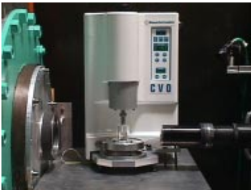
Figure 1.7.: Experiment installed at the Institut Laue-Langevin. the stress controlled Bohlin CVO rheometer on the instrument D11. This allows to obtain SANS data from samples under various shear conditions: controlled shear stress or controlled shear rate, simple shear, oscillatory shear, and creep. The rheological data are obtained simultaneously. [ZLR99]
