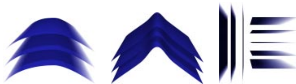
Figure 6.13.: The three tilt boundaries found by Gido et al. [GT94], the chevron, the \Omega -type and the T-junction.
