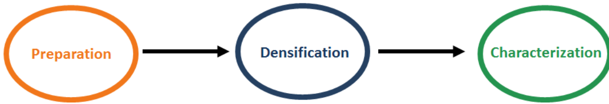
Figure 1.11: In the field of thermoelectrics the conventional processing can be divided into three parts, (i) the preparation of the powder, (ii) the densification into pellets and the subsequent (iii) characterization. In case of nanoparticular compounds the preparation and the consolidation step are exceptionally challenging.
