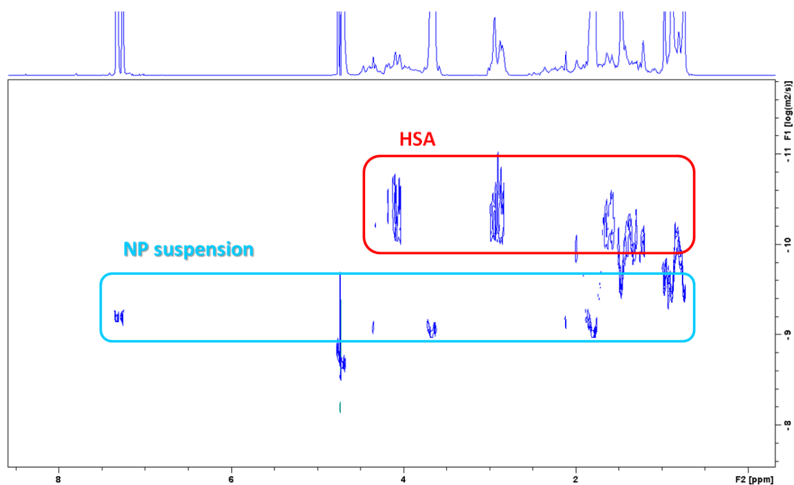
Figure 4.2.28 DOSY spectrum of a mixture of SDS-stabilized PS-NPs and HSA with signals assigned to each species.
