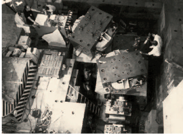
Figure 2.3: The first low energy K^- -beam for hypernuclear physics was build at CERN. In order to achieve a pathlength of 10 meter pions and kaons depending on their stopping power in a fluid absorber were partially separated in the middle of the chicane
