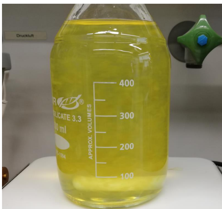
Figure 5.34 Large scale glyphosate degradation. (left) half liter scale photodegradation of 1 g of glyphosate in water.
