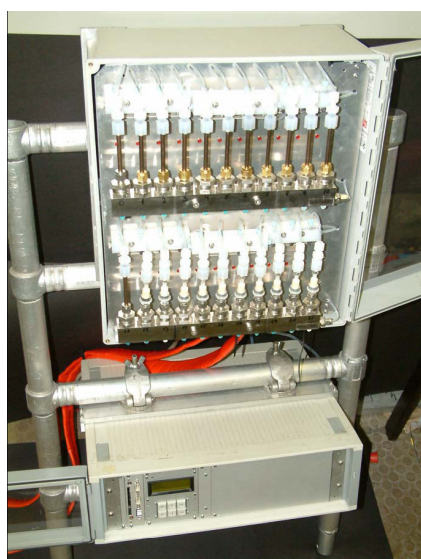
Figure 2.2.3.1 Automated cartridge sampling device with control unit
