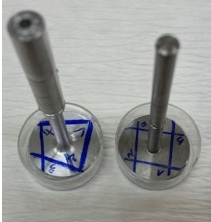
Figure 6: Picture of the sample holder with the four different lines for measuring the thickness of the HCP cores.
