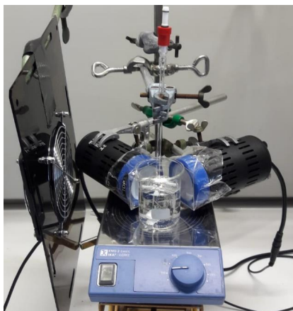
Figure S3. Setup for the irradiation experiments using two blue LEDs.
