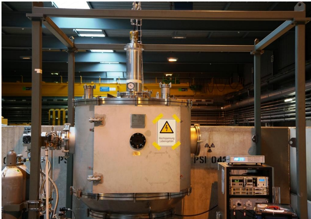
Figure 5.18: Photograph of HVtest. The whole setup is mounted on a platform for flexible positioning. To operate HVtest only pressurized air, electricity, and local area network need to be connected to the platform.
