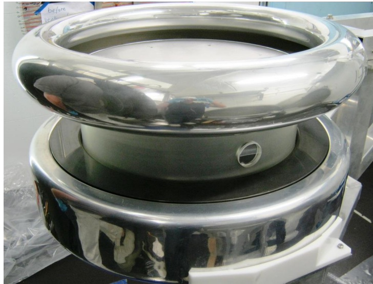
Figure 2.20: The precession chamber before installation into the experiment. Two corona rings are mounted onto the electrodes for high voltage performance.
