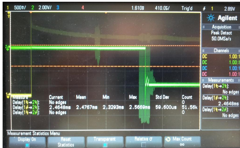
Figure 4.18: A function generator turned the relay on and off, used for the \pi/2 -pulse of the UCN, every second. The time delay between the signal of the generator and the actual opening or closing was measured for more than 50000 cycles. The relay needs (2.4767 \pm 0.0003) ms to close (shown here) and (1.3885 \pm 0.0001) ms to open.
