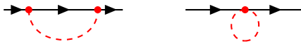
Figure 3.4.: One-loop Feynman diagrams with virtual ALP exchange (red dashed line) contributing to the fermion self-energies. The fermion line represents a quark or a charged lepton.
